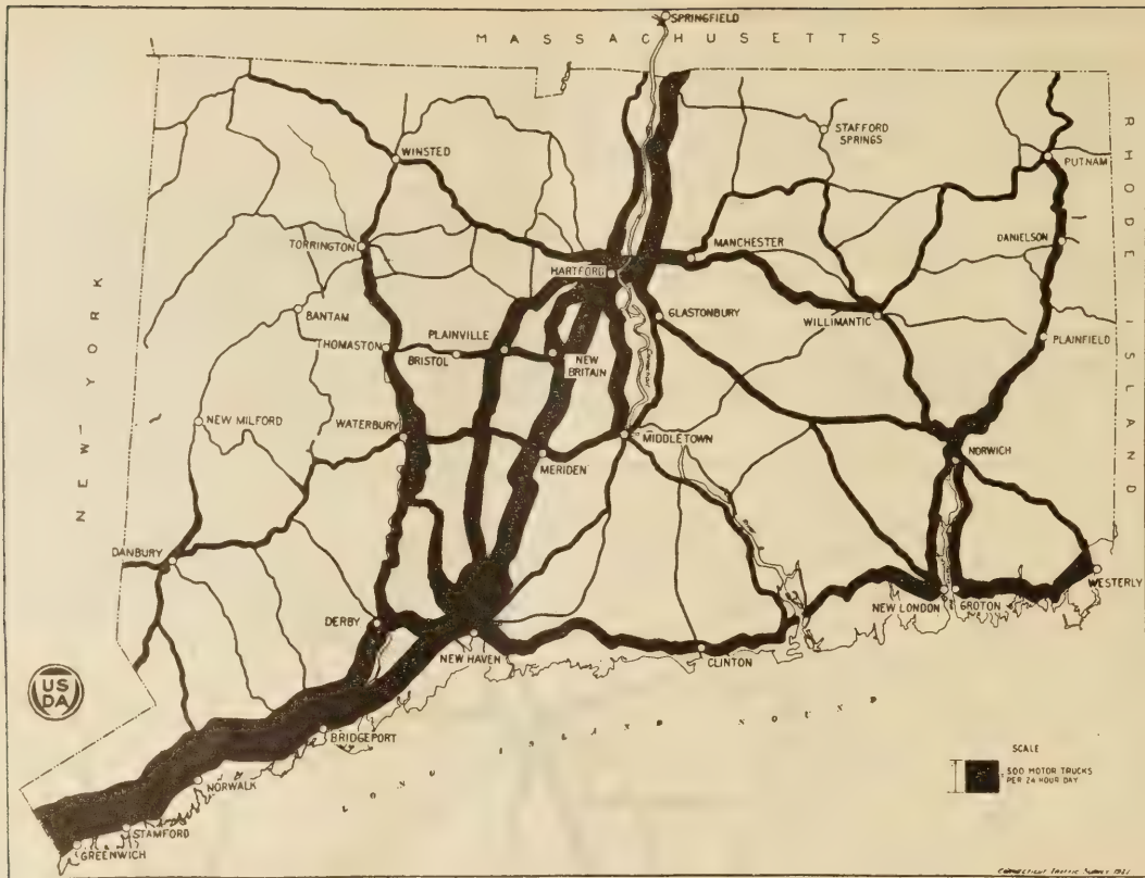
Fig. 3.—Average daily movement of motor trucks on the Connecticut highway system. Width of lines indicates density of traffic.
